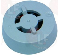
3120475 ADJUSTER FOR INLET ROBERTSHAW ORANGE flow rate 8 L/min - tolerance +/- 15%
