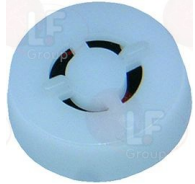
3120499 ADJUSTER FOR OUTLET ROBERTSHAW BLU flow rate 1.2 L/min - tolerance +/- 25%
